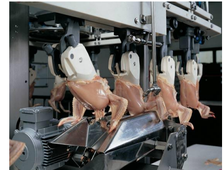
Stork's FHF-XB front-half deboning line is at the core of our business and impressed visitors at the 2009 IPE in Atlanta
