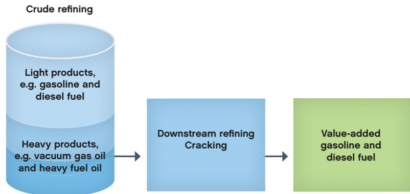
**i** Heavy refining fractions are converted into value-added, low-emission traffic fuels.
