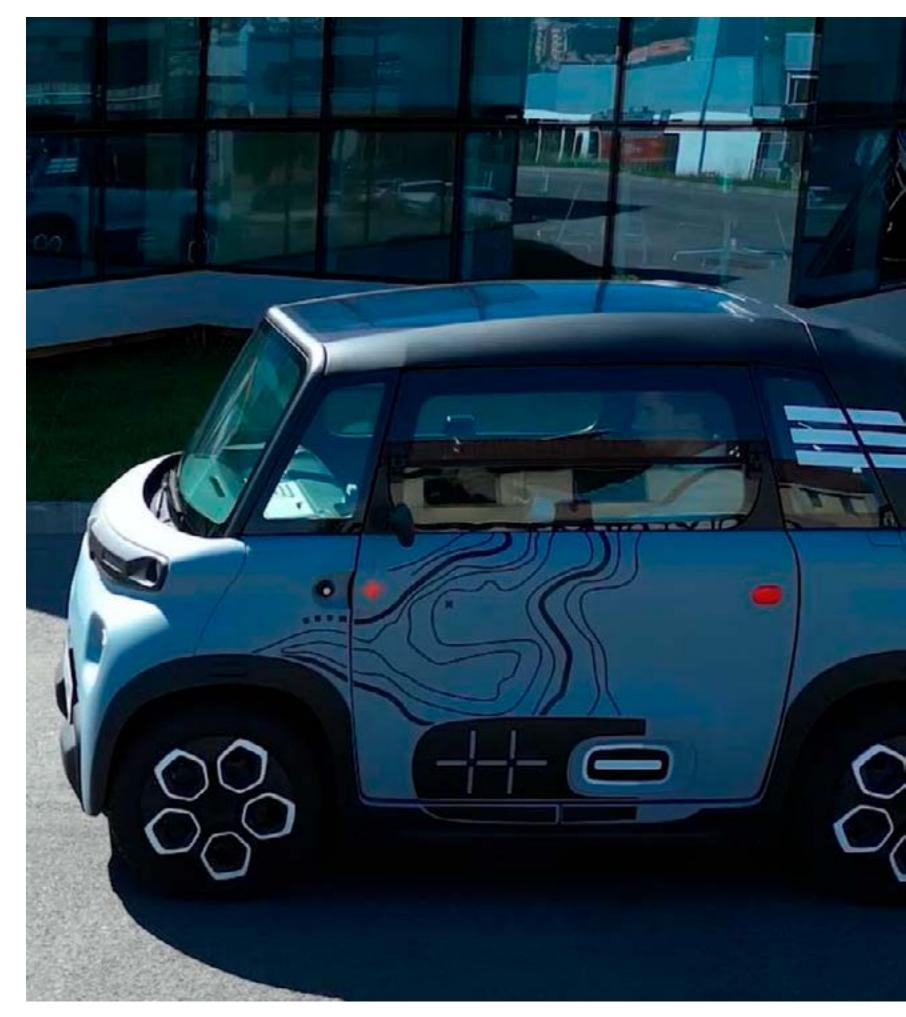
Together with Simoldes Plasticos, Valoe manufactured prototypes of a lightweight polymer-based solar roof for Stellantis. Valoe's composite solar roof strengthens the structure of the car, is lightweight and mechanically robust and can be brush washed.
