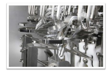
The VO-20 RS opening machine has set a new standard in poultry processing, offering reliable opening cut and preventing intestine damage and bare breast tips.
